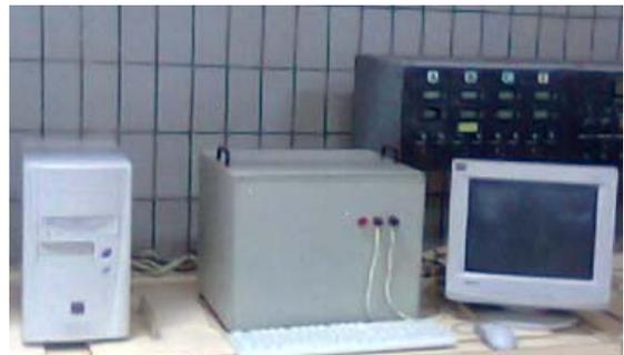
Fig.1. Computer controlled pulse-reversed current source
